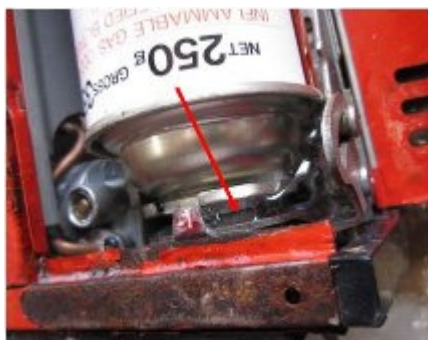
Position of gas leak
