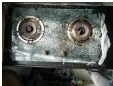
Broken glass panel of built-in gas hob
